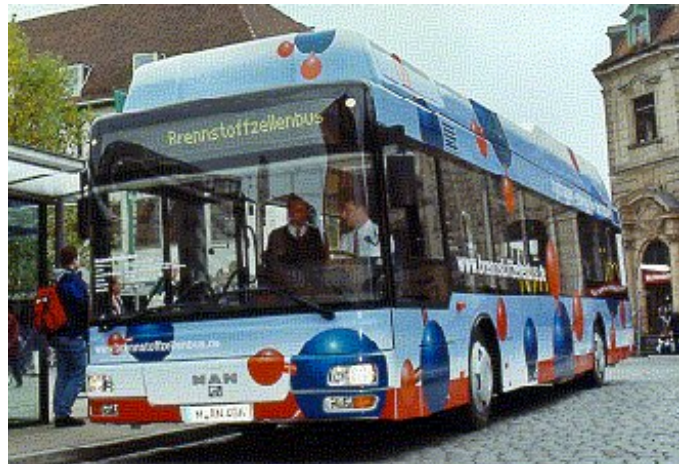
Fig. 5: MAN's first fuel cell bus in operation in Erlangen, Nuremberg and Fürth, powered by four fuel cell stacks;
