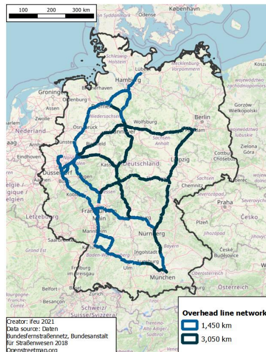
Figure 2: Assumed overhead line network for catenary trucks (light blue roads are part of the 3,050 km basic network)
