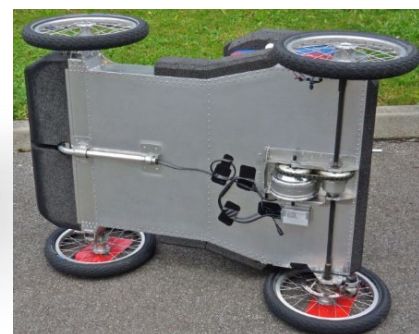
Fig. 2 Platform with integrated E-bike motor and chain to differential
