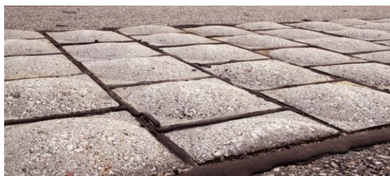
Figure 2 The rumble strip test track built by special cobble stones with a diameter of 100 mm and a height of ~15 mm.
