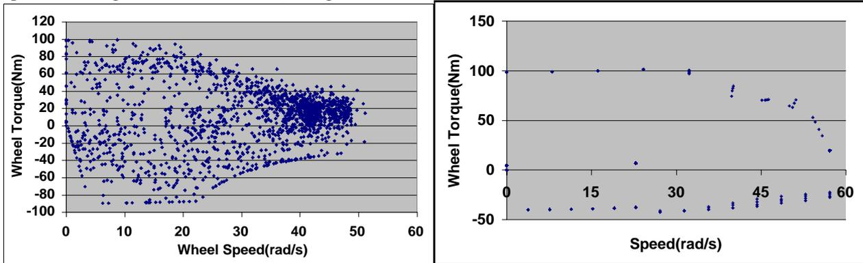
**Figure 3: Distribution of operating points for On road measured cycle (left) and ECE 47 (right)**
