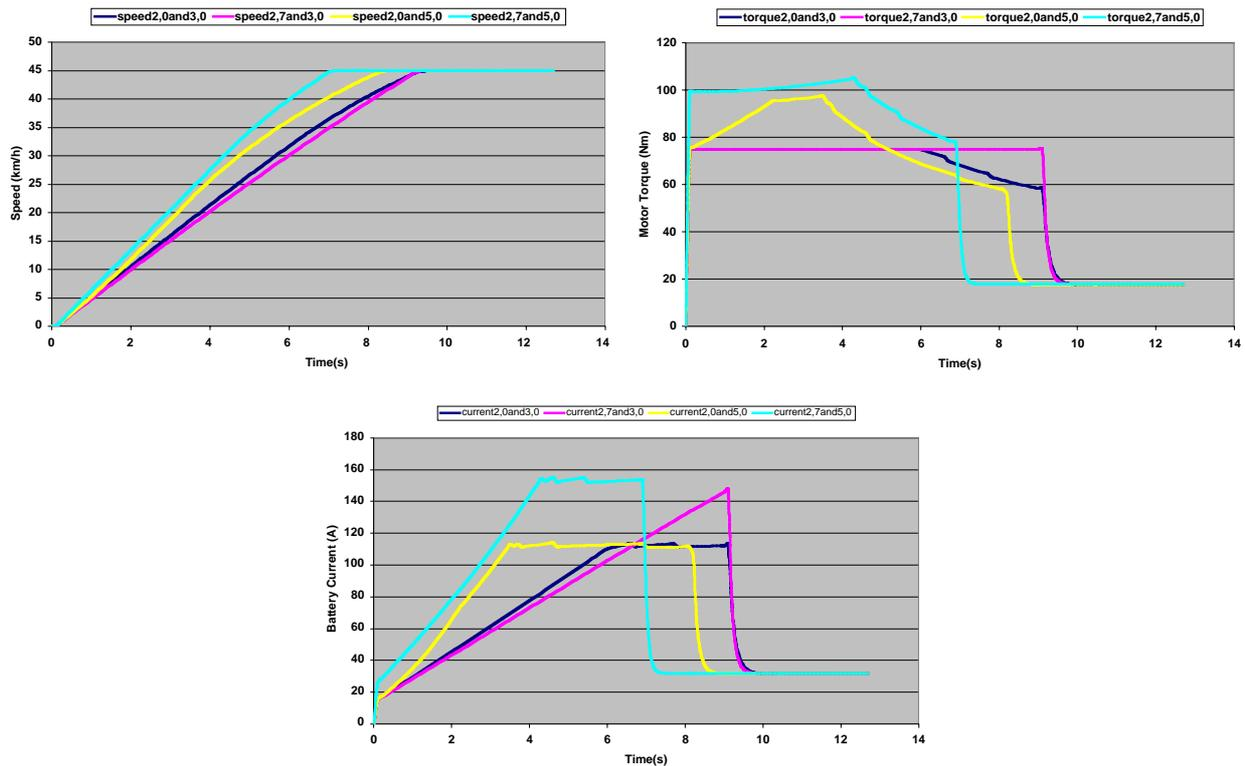
**Figure 5 : Simulation results of the acceleration test**
